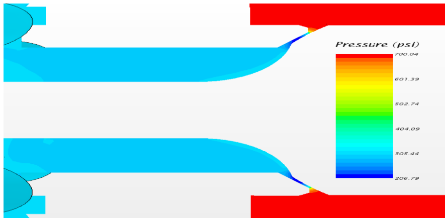
Figure 5.48. Unsteady state pressure scalar - type A- gap 0.005in, time-step 0.08S.
