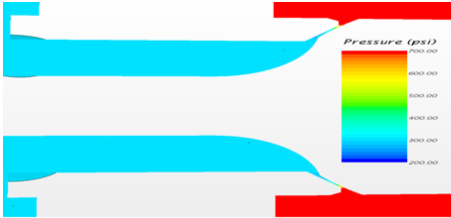
Figure 5.7. Steady state pressure scalar - type A- gap 0.002in.
