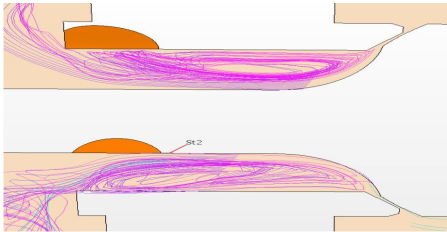
Figure 5.53. Unsteady state streamline plot at the expansion area, gap 0.002in, valve type A, time-step 0.004S.
